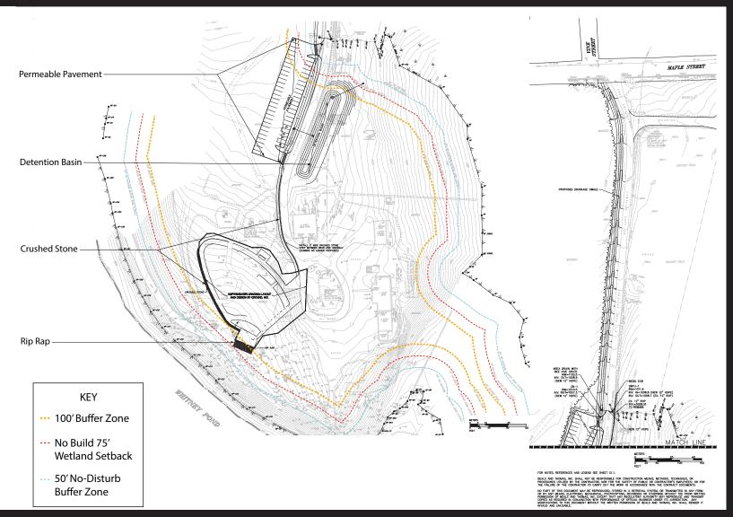
Storm water and runoff has been designed to minimally impact the site by using permeable paving, and thoughtfully placed detention basins, crushed stone strips and rip rap.
