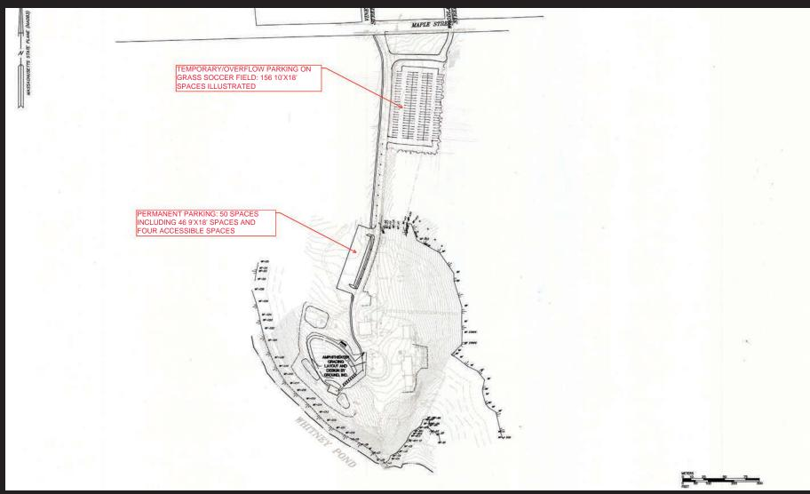
50 Permanent (4 accessible) parking spots provided adjacent to the accessible sidewalk leading to the amphitheater plaza. 156 Temporary / overflow spaces provided on the ball field
