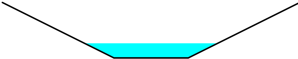
Reach PRB: Perimeter Swale
